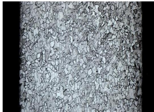
Figure 3. Metallographic image of 1.0347 sheet with 100X magnification
