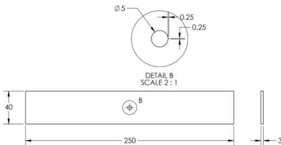
**Figure 3.** Schematic drawing of the thermal fatigue test specimen (in mm)
