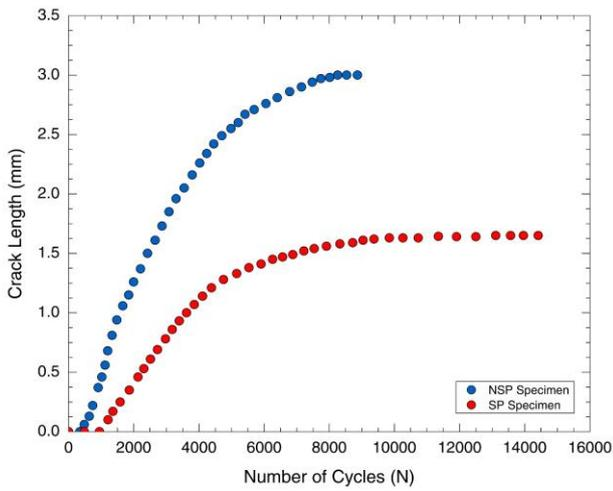
**Figure 10.** The thermal fatigue life curve for crack growth
