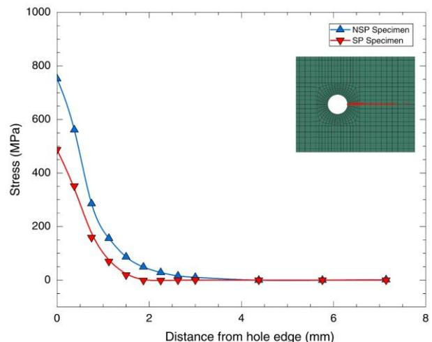
**Figure 9.** Normal stress (i.e. along the Y direction) distribution on the crack propagation path of two specimens
