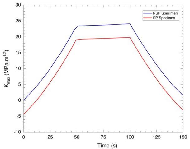
**Figure 12.** The simulated SIF for NSP and SP conditions against (a) the crack length, and (b) the cycle time at the crack length of 1 mm
