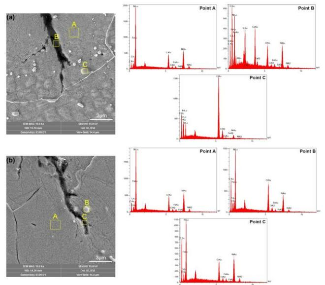
**Figure 20.** EDS point analysis; (a) NSP specimen, and (b) SP specimen
