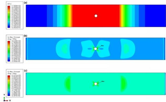
**Figure 8.** FE simulation results at the maximum load condition in MPa: (a) nodal temperature distribution; (b) normal stress (i.e. along the Y direction) of the NSP specimen; (c) normal stress (i.e. along the Y direction) of the SP specimen
