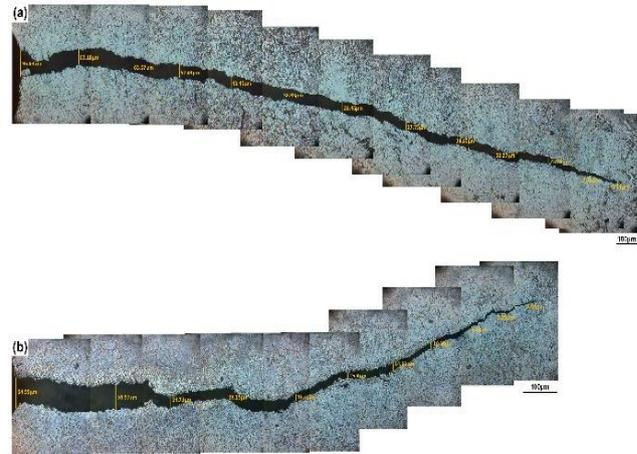
**Figure 17.** Optical micrographs of the thermal fatigue crack: (a) NSP specimen, and (b) SP specimen
