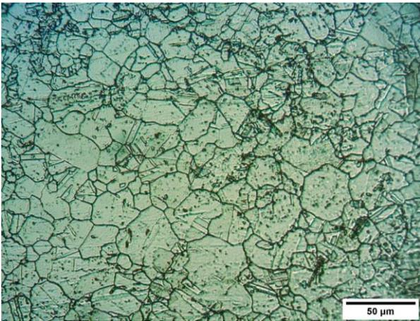
**Figure 2.** Optical micrograph of the microstructure of Ni75 alloy
