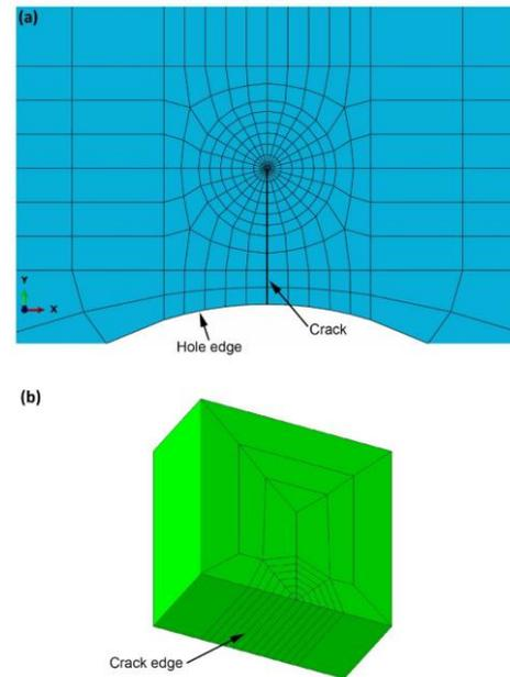
**Figure 7.** FE model (a) thermal fatigue specimen meshed geometry with a crack, and (b) the element s04\_t35x1 schematic
