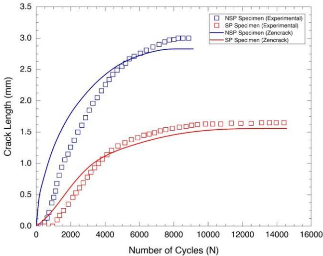
**Figure 14.** Comparison between experimental and FE crack growth results for NSP and SP conditions
