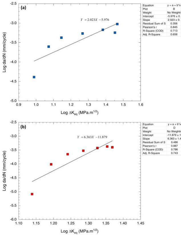
**Figure 13.** da/dN versus ΔK<sub>eq</sub> in the logarithmic scale and the lines of best fit made to the data for: (a) NSP specimen, and (b) SP specimen
