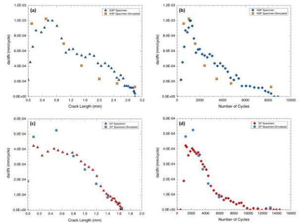
**Figure 16.** Comparison of the experimental and simulated crack propagation rates versus crack length and the number of thermal cycles for: (a and b) NSP condition, and (c and d) SP condition
