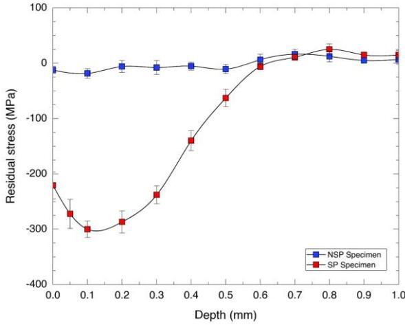
**Figure 5.** XRD residual stress measurement on the NSP and SP thermal fatigue test specimens
