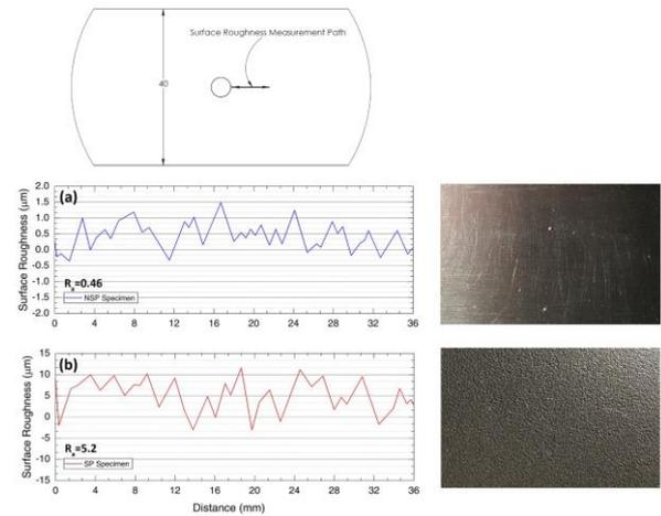
**Figure 4.** The surface roughness of the specimens: (a) NSP specimen; and (b) SP specimen
