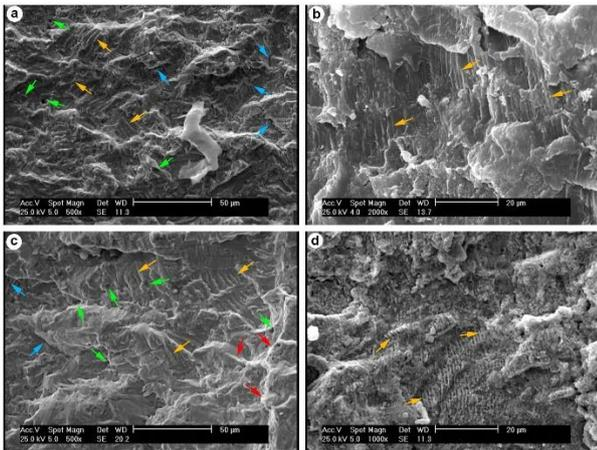
**Figure 22.** SEM images of the fatigue fracture features and the morphology of striations: (a and b) NSP specimen, and (c and d) SP specimen
