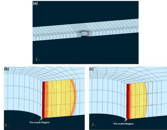
**Figure 15.** Simulated crack growth profiles: (a) specimen cut view, (b) NSP specimen, (c) SP specimen
