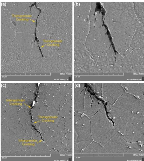
**Figure 19.** SEM micrographs of the thermal fatigue crack tip: (a and b) NSP specimen, (c and d) SP specimen
