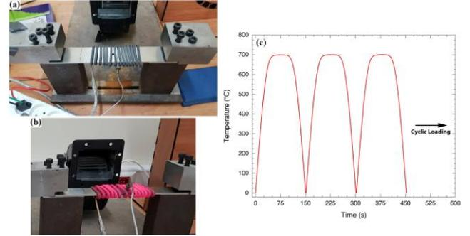
**Figure 6.** Experimental set-up for thermal fatigue tests (a) before heat up, (b) after heat up, (c) Applied thermal cyclic loading pattern
