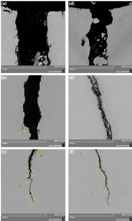
**Figure 18.** SEM micrographs of the thermal fatigue cracks: (a, b and c) NSP specimen, and (d, e and f) SP specimen
