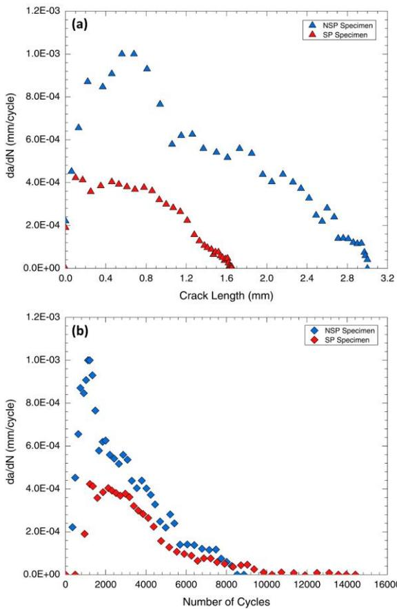
**Figure 11.** The crack propagation rates for the NSP and SP conditions against (a) the crack length, and (b) the number of cycles
