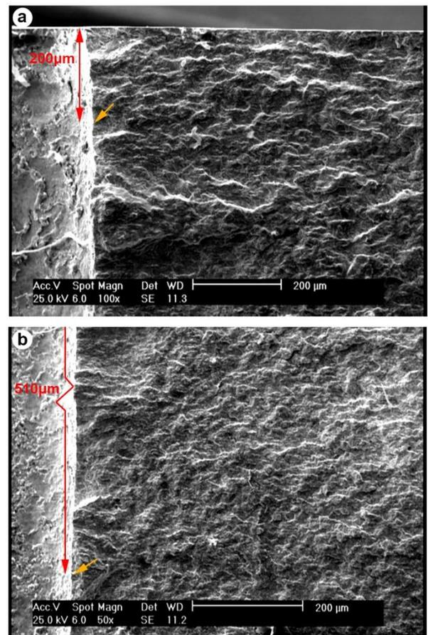
**Figure 21.** The fractured surface of the test specimens: (a) NSP condition, (b) SP condition
