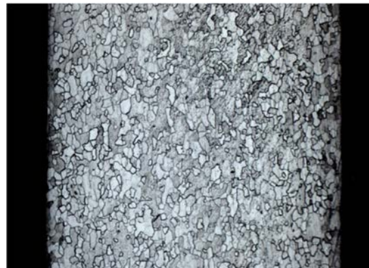
Figure 3. Metallographic image of 1.0347 sheet with 100X magnification
