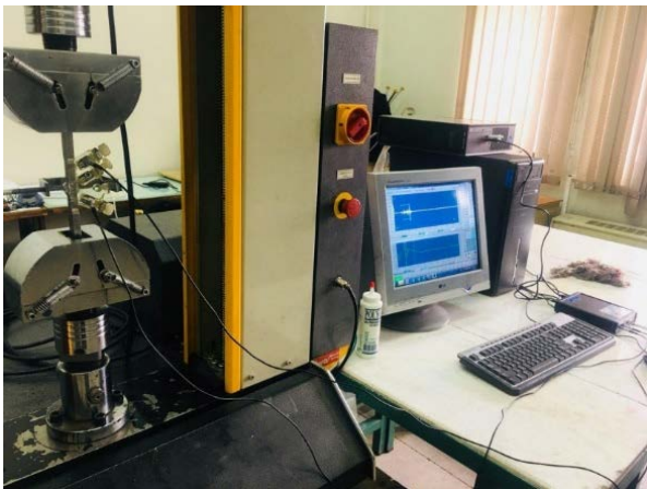
Figure 8. A view of measuring the acoustoelastic coefficient for steel 316L
