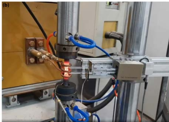
Figure 3. LCF test: a) specimens schematic (in mm); b) test setup
