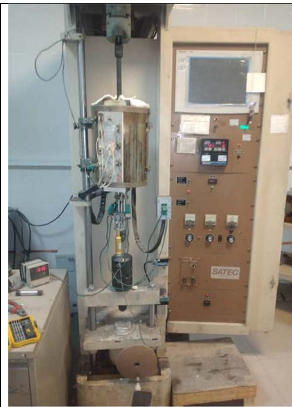
Figure 8. Test setup apparatus used for the creep testing
